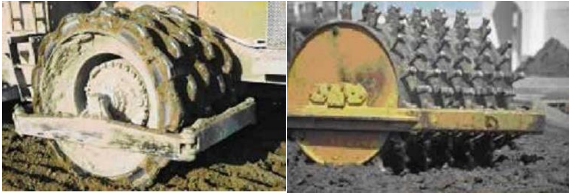
Fig.6 Sheepsfoot (above) & padfoot (below) rollers
